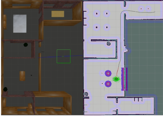
Fig. 5. Simulated experimental results: Gazebo simulator environment (left) and the navigation stack using Dijkstra's algorithm and DWA planner (right).
